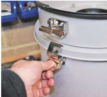
▲ High-quality toggle clips secure the Hepa and motor housings firmly
